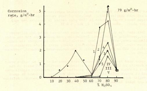
Corrosion rates at room temperature in 100-hr test in sulfuric acid of various concentrations (Arabic numerals) and 164-hr test in 80% sulfuric acid (Roman numerals) 1 and I - unalloyed titanium; 2 and II - 1% platinum alloy; 3 and III - 2% platinum alloy; 4 and IV - 1% palladium alloy; 5 and V - 2% palladium alloy.
