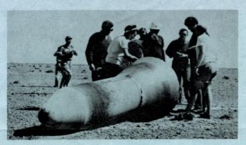
The re-entry vehicle for President Charles de Gaulle's ICBM Force de Dissuasion test rocket, the SAPHIR, is shown shortly after recovery after the most recent flight of the vehicle on October 9 (SPACE Daily, Oct. 8, 14 & 19). The SAPHIR is being used as a test vehicle for the MINUTEMAN-(SSBS) and POLARIS-type (MSBS) ballistic missiles which France is hope-
