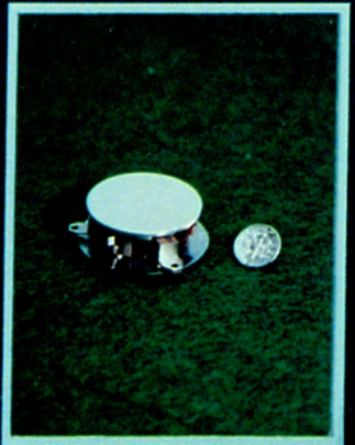
Assembly of a flight fold mirror invar flexure and bezel. Electrostrictive ceramic actuators within this structure provide tip/tilt adjustments up to ±1 milliradian in each axis.
