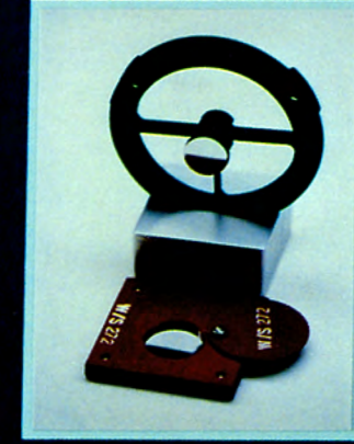
One of three flight WFC Cassegrain relay secondary mirrors, mounted on its support spider. An image of the aberrated Hubble primary mirror is projected onto the surface of these relay secondaries, which are figured to cancel the Hubble aberration.
