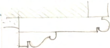
← NOTE SQ. PEG AT SASH CONNECTION
