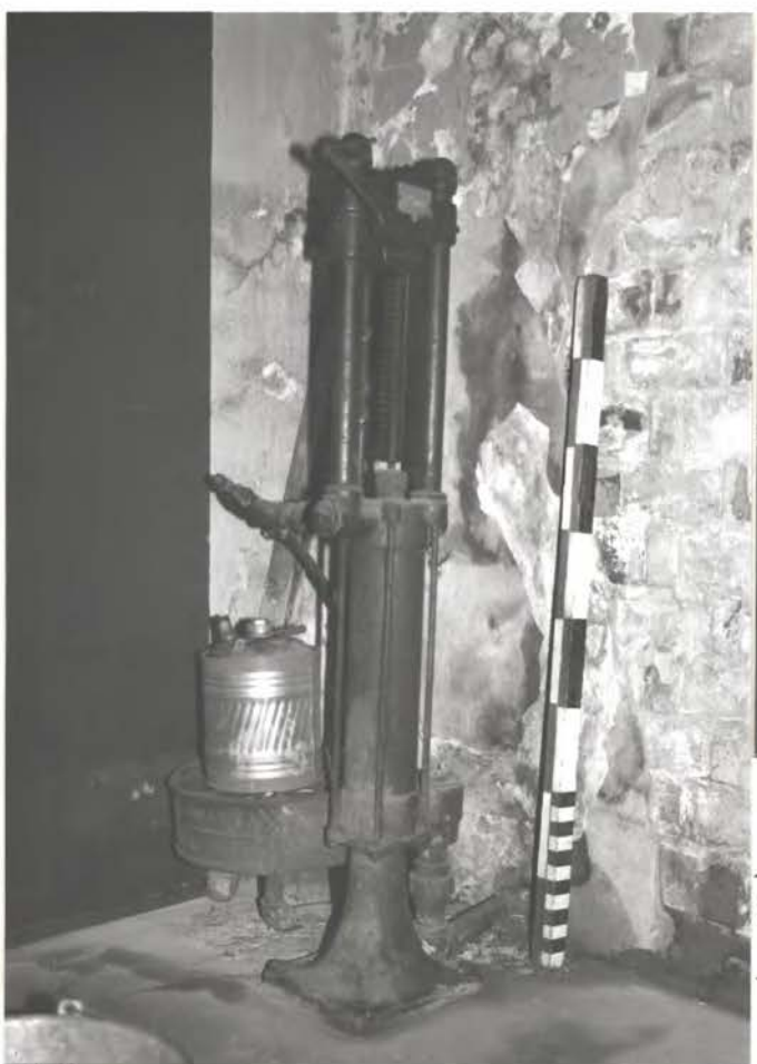
Kerosene pump (tank is buried) - kerosene was main lt. source in early 20th c.
