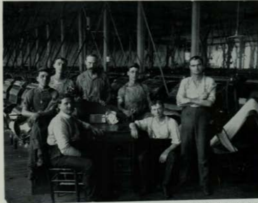
(Photograph property of Mrs. Willie Vann) This room contained 400 small cards, known as "railroad" cards. Weights seen hanging off the cards on the left hand side of the picture could be added to or taken away as the case warranted, if the lap were light or heavy.
