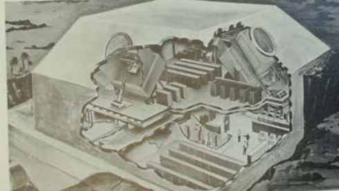
MISSILE SITE RADAR —This is an artist's concept of the Missile Site Radar (MSR) for the Sentinel Ballistic Missile Defense System. The MSR is a multi-function, phased-array radar which will detect and track incoming enemy missiles and guide Sparrow or Sprint interceptor missiles to destroy them. (U.S. Army photo)
