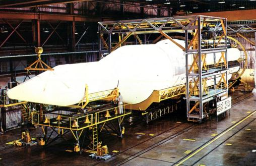
i The first flight configuration of the giant Saturn C-1 rocket is seen at the George C. Marshall Space Flight Center, N.A.S.A. Huntsville, Ala. The C-1 will be capable of placing about 10 tons into low earth orbit.
