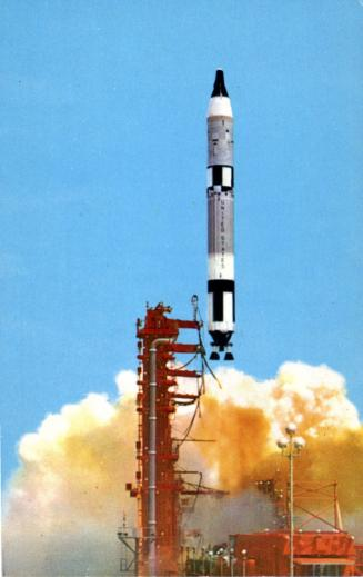
Gemini-Titan 1 lifting off launching pad on its maiden voyage, testing spacecraft and vehicle. The Gemini is the first of NASA's two-man spacecrafts.
