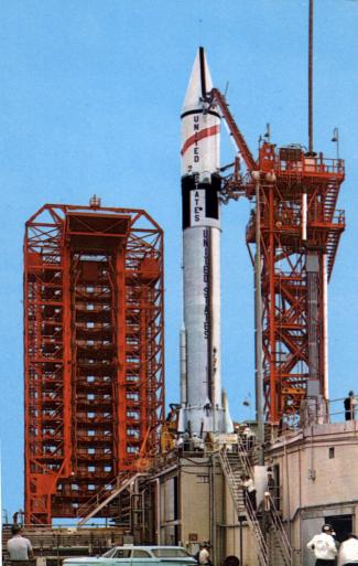
Centaur II, our first space vehicle to use liquid hydrogen as a propellant, undergoes prelaunch tests.
