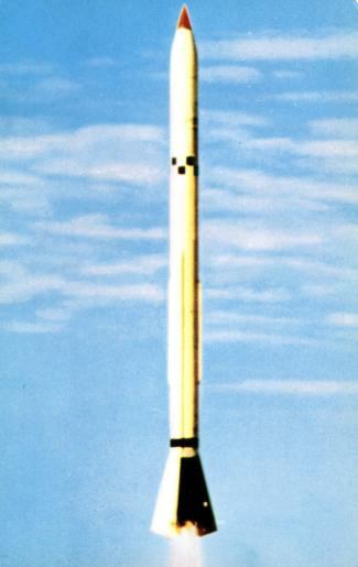
A member of the Army missile family used in support of ground combat operations, the Corporal, equipped with either an atomic or conventional type warhead, is a surface-to-surface guided missile capable of engaging tactical targets far beyond the range of conventional artillery. A powerful rocket motor propels the missile through space, at several times the speed of sound.
