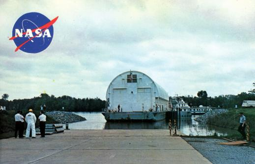
Saturn rocket booster barge at dock on Tennessee River. Barge is used to carry boosters from MSFC at Redstone Arsenal, Ala., to NASA-Kennedy Space Center, Fla., for launch.
