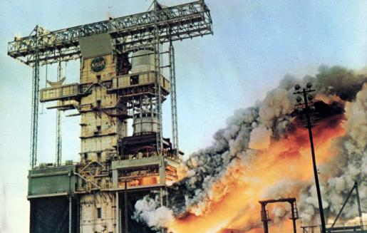
An F-1 engine, generating 1.5 million pounds thrust, is captive fired at the NASA-Marshall Space Flight Center, Huntsville, Alabama. The liquid oxygen/RP1 (kerosene) engine is used on the Saturn V booster.
