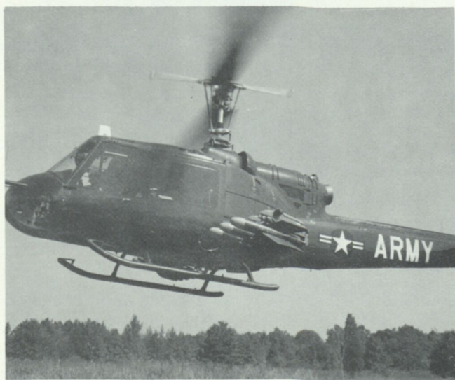
M22 —A subsystem consisting of a boom assembly on each side of the helicopter which mounts three SS-11 missile launchers on each boom. The system is effective against armored vehicles and other hostile targets.
